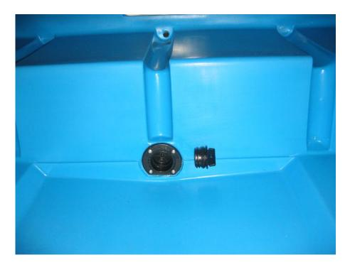
1 x drainage bung is located at the stern, on the back edge of the keel. This is only removed if it is necessary to drain water from between the hull skins.
